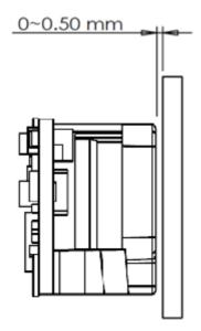
If the window is required to be in a tilted position, the above distance requirements should be met and tilt angle should ensure no reflections back into the lens.
