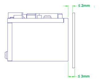
If the window is required to be in a tilted position, the distance requirements above should be met and tilt angle should ensure no reflections back into the lens.
