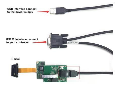
PS: If you use the scanner with USB cable (USB-HID KBW) firstly, and want to change it with RS232 cable, please scan below setting code on USB-HID KBW mode before connect the RS232 cable.
