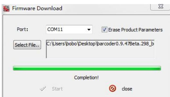
When it is completed, you need to re-connect the scan engine with computer.
