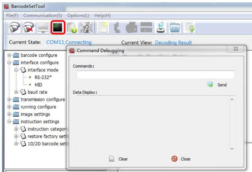
2. Input the command and click send button. (you can find the command list from [Protocol Map.xls](#) under the SDK package.)
