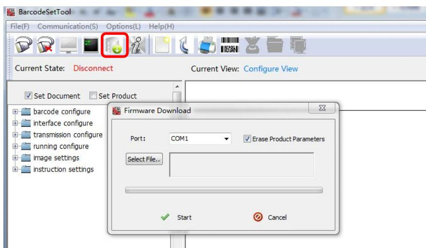
**2、Select the corresponding Com port and firmware, press 'start':**
