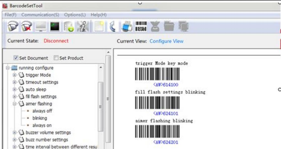
(2), Click the “Merge Setting Codes” button to generate a new setting barcode. Scan this only one new bar code to finish the setting of all the above listed bar codes.
