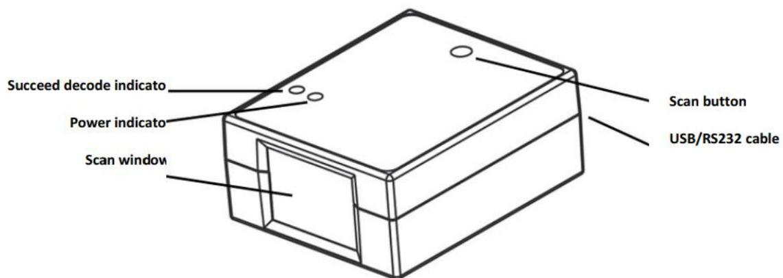
\*Kindly note the reader is default set as Sense Mode which can read barcode automatically, so pressing button is not necessary.
