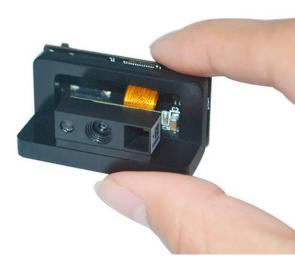
The RT214C is an OEM barcode scanner module launched in 2021. It's outstanding at its excellent bar code read performance, lower power consumption. Also outstanding in its compatibility with some traditional barcode scanner modules in terms of size and fix screws.
