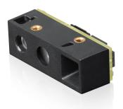
RT214D scanner engine is designed to be small, cost-effective, and energy-efficient, making it an ideal choice for most kinds of embedded use for common 1D/2D barcode reading.
